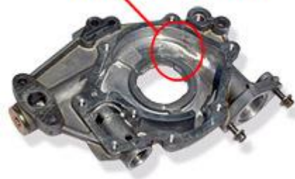
Crack in Factory Housing
